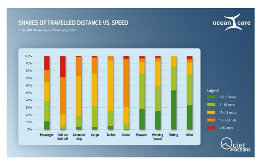
Roll-on roll-off vessels have the smallest percentage of distance travelled at speeds below 10 knots, which are considered safe for marine biodiversity in terms of collisions. They are followed by cruise ships which travel most of their journey at speeds between 15-20 knots. The majority of fishing vessels travel at safe speeds for approximately 85% of their route, therefore a speed limit would have minimal influence on them.
