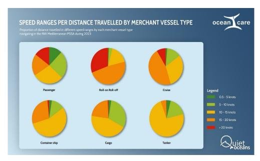
The graph illustrates the speed at which the six main types of merchant vessels travel. It shows that all of them cover the majority of their distances at speeds exceeding 10 knots, with roll-on/roll-off and cruise ships exceeding 15 knots. It is noteworthy that the best available scientific evidence indicates that the likelihood of a collision causing a fatal impact on a whale is extremely minimal if the speed of the vessel remains below 10 knots.
