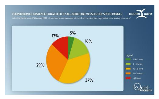
Merchant ships travelling at speeds exceeding 10 knots account for 79% of the total distance travelled by these ships in the NW Mediterranean PSSA during 2023. The majority of the distance covered (37%) occurs within the speed range of 10-15 knots, making it quite feasible to minimise its impact on marine life by just dropping a few knots.
