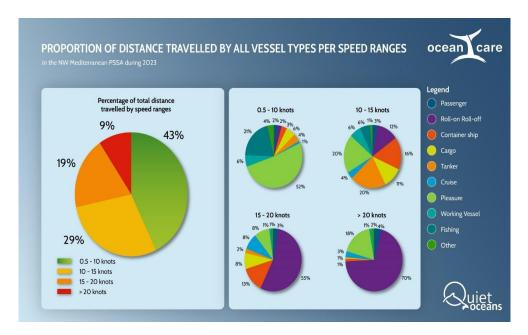
When considering all types of boats together (represented at the left side of the graph), and despite the statistical effect that occurs when including pleasure boats and fishing vessels in the calculation which tend to travel at speeds below 10 knots for a significant portion of their journey, it is evident that 57% of the total distance navigated by all vessels in the PSSA in 2023 was travelled at speeds greater than 10 knots, which entails serious risks for fin whales and sperm whales.
